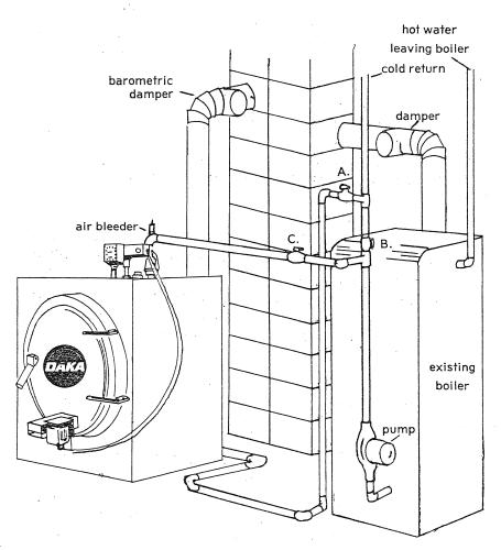
NOTE: B-1000 must be kept at least 3' fron any combustible material.
