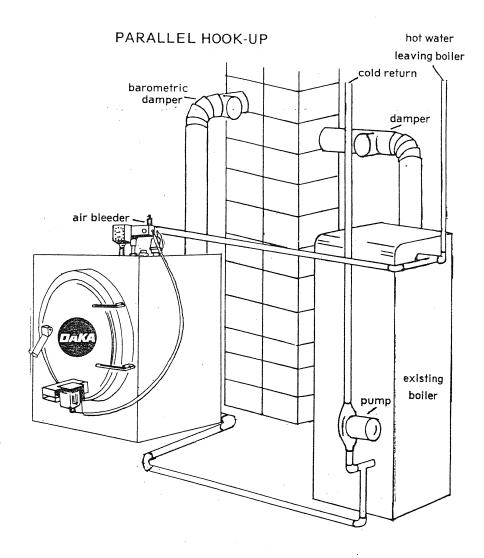
NOTE: Check existing boiler for extra tapped holes and hook-up as pictured, if taps are not available, T into existing pipes at boiler.
